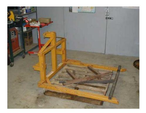
First he started with a basic frame from another item, then mounted the top dresser from a Cushman and hooked it up to the tractors remote hydraulics.
